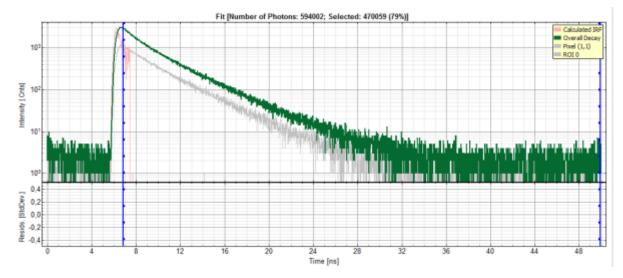
• In the decay form on the lower left, select n-exponential reconvolution as fitting model.
