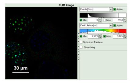
• Set the intensity scale from 0 counts – 200 counts and the lifetime scale from 0 to 5 ns.
