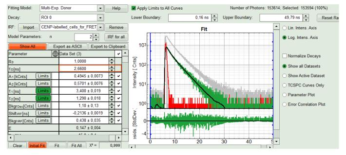
• In the Fitting panel, set the parameters Bkgr<sub>Dec</sub>, Shift<sub>IRF</sub> and Bkgr<sub>IRF</sub> constant by removing the mark. Set the background of the decay to 0.
